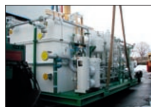
Lubricating oil unit for compressor station with BOLLFILTER Duplex type BFD-P
